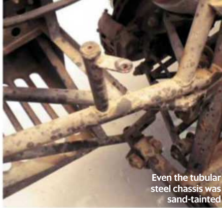
Panels are bonded to the chassis, so were left in situ
