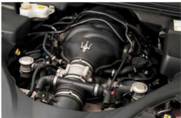
The F136 V8 engine was a joint Maserati/Ferrari project, built by the latter. Quattroporte V is powered by 4244cc or 4691cc versions, with 395-434bhp
