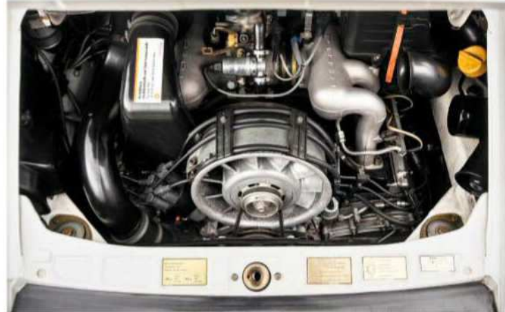
Minus turbo, the Porsche flat-six delivers its power smoothly
